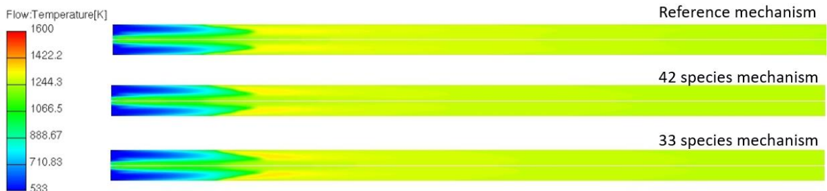
Figure 3. Comparison of temperature field obtained with three mechanisms for case of gradual combustion.
