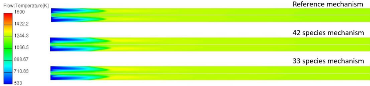
Figure 5. Comparison of temperature field obtained with three mechanisms for transition case between gradual and fast combustion.
