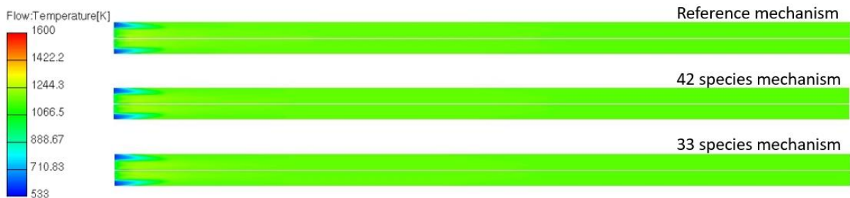
Figure 4. Comparison of temperature field obtained with three mechanisms for case of fast combustion.
