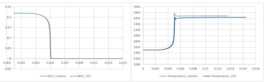
As a first real case, the simulation of the premixed ammonia burner described in the paper of Kobayashi and associates was performed. For this geometry there is a large body of simulation data obtained by using LES approach for turbulence modelling. The authors from literature used Miller's mechanism, whereas in the present simulation the reduced mechanism from Mathieu developed at IST was employed.
