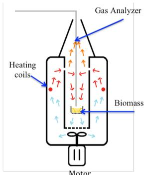
Figure 1: Cross section view of the furnace.
