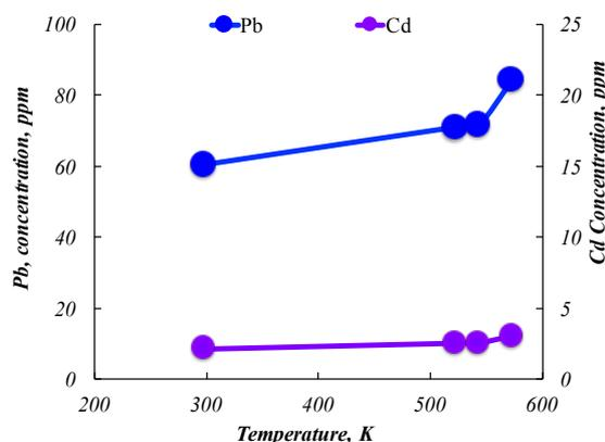
Fig. 3: Concentration of Pb and Cd in the chars produced different final temperatures.
