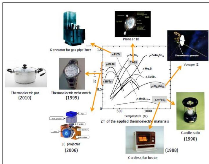
Fig. 2 History of typical applications of thermoelectric power generation [15].
