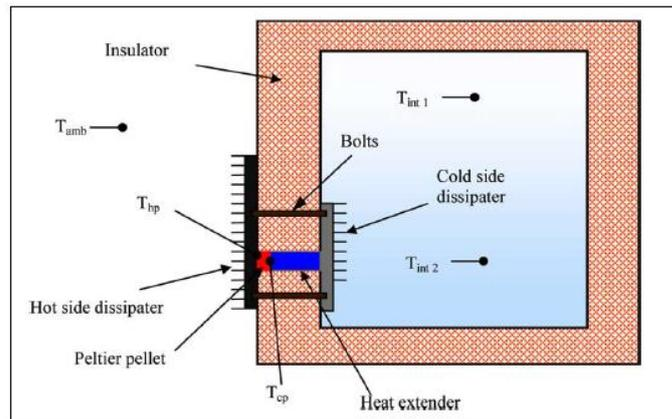
Fig. 1 Thermal sketch of the thermoelectric refrigerator [14].
