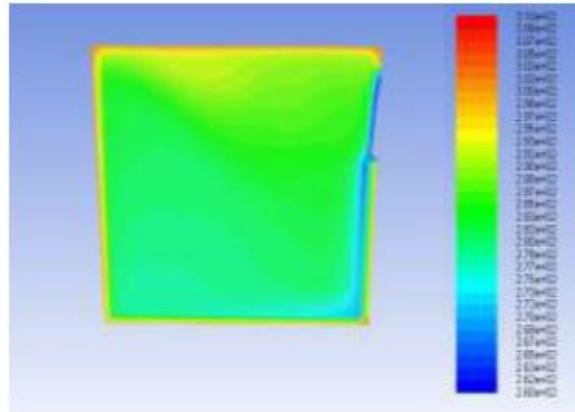
Fig. 3 Temperature distribution of Peltier power (200 W)
