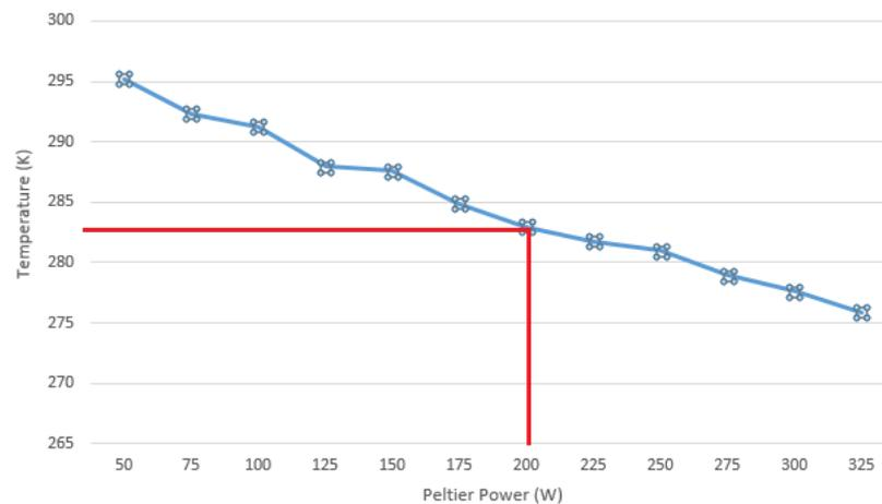
Fig. 4 Optimal temperature distribution associated with Peltier power.
