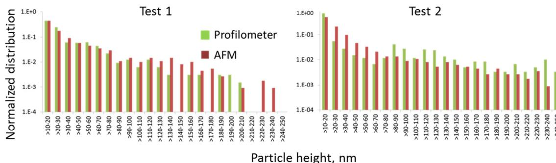
Fig.2 Normalized distributions of the heights of the particles/aggregates found by surface profilometer compared with those estimated by AFM measurements.
