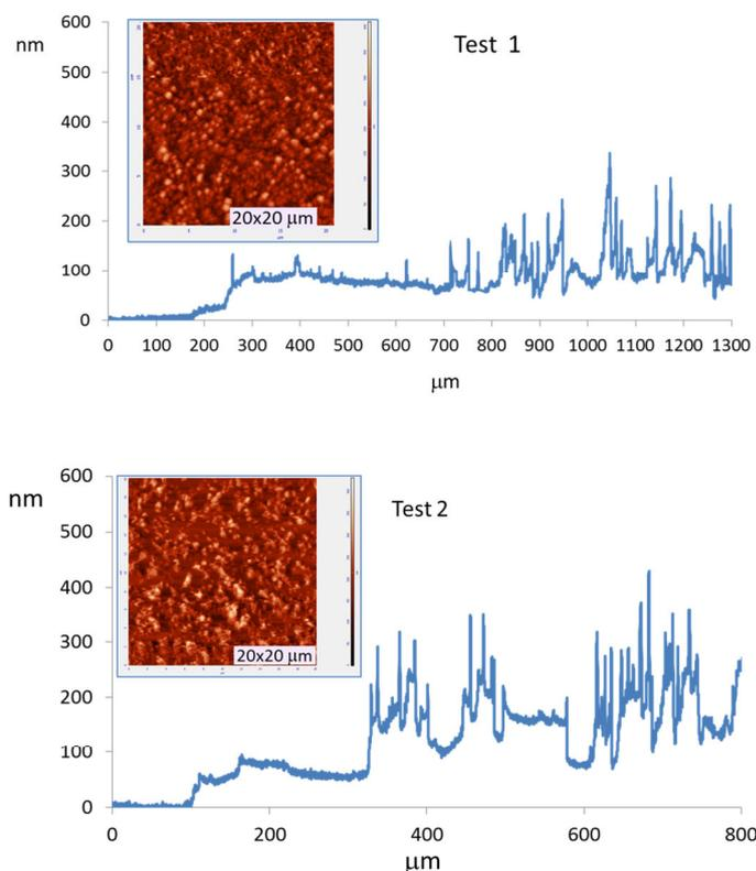
Fig. 1 Height profiles measured by profilometry of particulate carbon deposited at 8mm HAB with 240ms deposition time (Test 1) and at 14mm HAB with 120ms deposition time (Test 2). AFM 2-D topological maps obtained on the same samples (insets).
