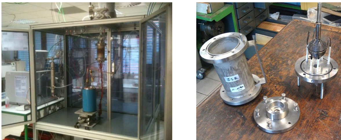
Figure 1. Pictures of the high-pressure JSR setup (left) and disassembled reactor's chamber (right)
